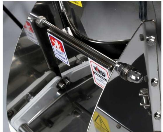
The peelers are normally delivered with a stainless coat. They can also be produced in a grey coated version. The catchers of the peeled skin and starch are always stainless. There is a movable inlet fixed on the machine, finished with a compact control switch with over-current protection, with protection features against twisting after a blackout, and with a STOP button.
